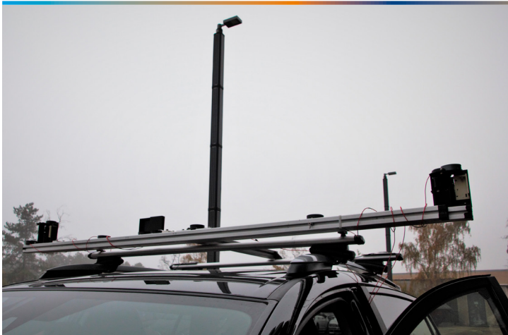
Quality measurements can also be carried out on road level. DOLL Quality Lab in Denmark has developed a universal roof rack with a range of sensors. Mounted on a car it enables driving through stretches of roads or entire cities, while making quality measurements of street lighting.
